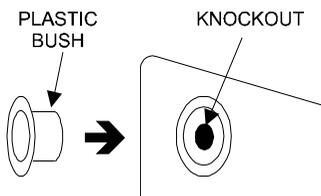
4. Ensure that all four plastic flanged bushes are in place and the rear enclosure is screwed tightly to the surface to prevent any water ingress through the punched holes.
