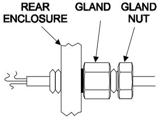
**IMPORTANT:** If only one gland entry is used, the BLACK blanking plug fitted to the second gland position must be left in place.
