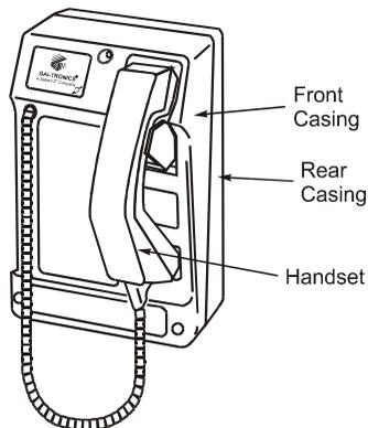
Commander is a family of rugged, weather-resistant telephones manufactured from moulded glass-reinforced polyester. A range of handset types and keypad configurations are available.
