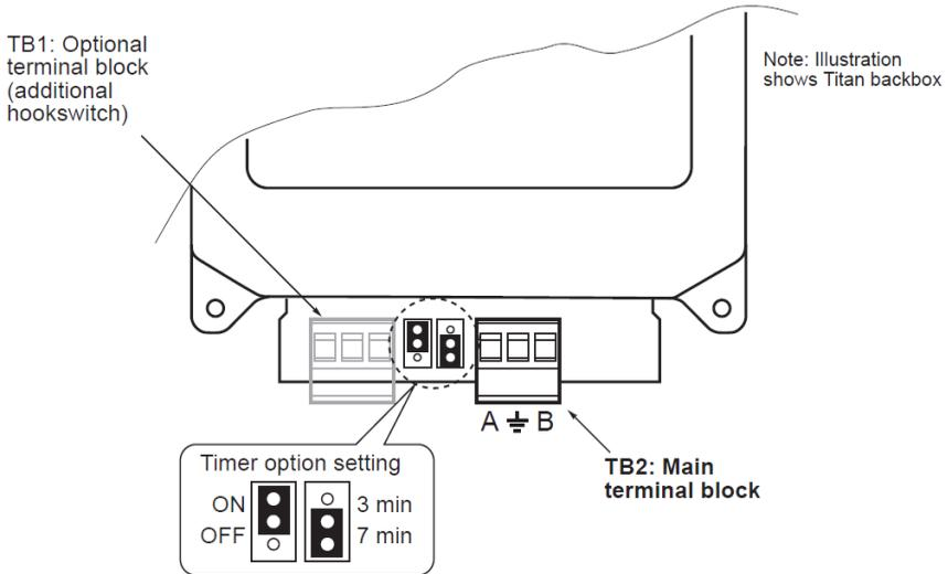
The centre earth terminal is intended for connection to a local earth to provide common mode protection from lightning transients. Particularly on Titan (metal bodied) telephones, **if this terminal is not earthed there is an increased risk that the telephone could be damaged by line-born transients.**
