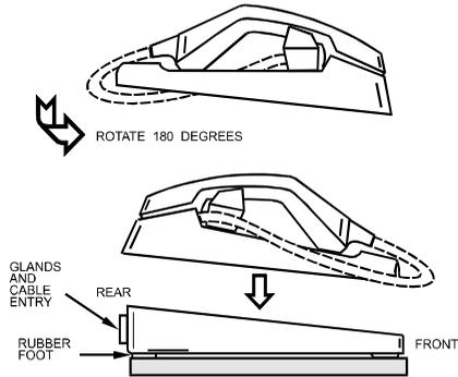
To provide a 'rake' for convenient operation, the Front Casing may be turned through 180° before it is fitted to the Rear Casing. Thus the cable entries are at the rear of the telephone.
