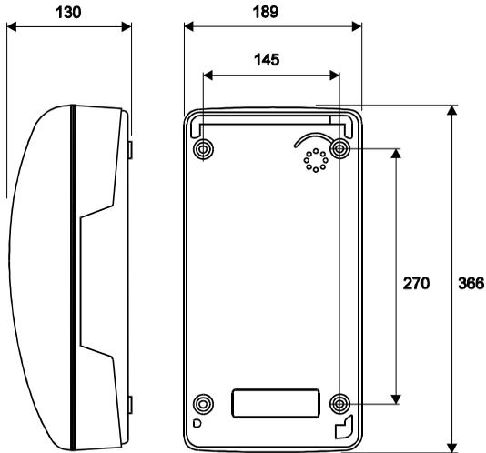
1. Using a suitable tool, punch out 4 holes in the rear enclosure, taking care not to damage or dislodge the plastic bushes. Only four of the eight holes are required - the outer ones are recommended. The inner holes are provided to be compatible with older-style mounting posts, and should be left intact if not used. If the inner holes are used they must be fitted with the supplied plastic bushes.
