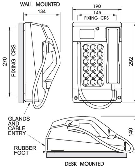
To ensure weatherproof integrity when wall mounted, external cables should enter the enclosure from the bottom via the 20mm gland entries provided.
